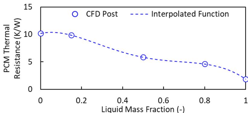
**Figure 8:** PCM Thermal Resistance Interpolation for Discharge Slope
